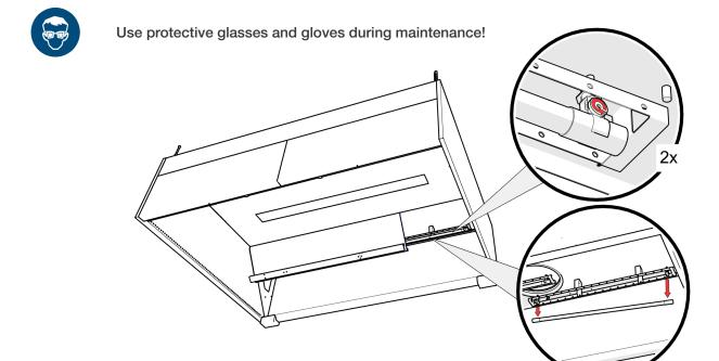
When the kitchen canopy has been serviced, the UV lamp and the UV control unit must be installed back into the canopy in the reverse order of how they were removed.
