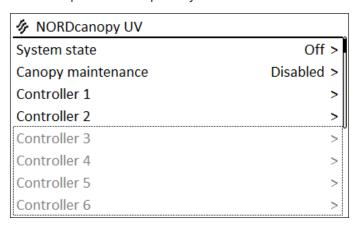
If you have several UV canopies in your kitchen, turning the system on/off is still done from the NORDcanopy UV menu under System state - it turns all the devices on and off.
