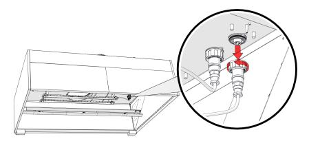
• After disconnecting the UV lamp from the plug, screw the cap of the bulb onto the open socket on the ceiling. The protective cap hangs from the socket.
