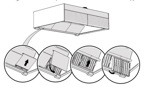
• Putting the HFK grease filters and UV protection shields back into the canopy.
