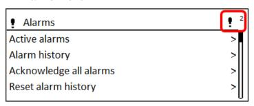
In the LCD alarm menu, you can check the active alarms and what alarms have been active. The number of active alarms is shown in the right corner of the main view.
