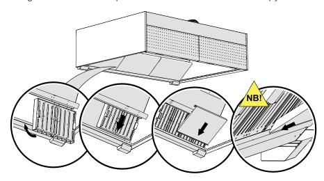
• Removing the grease colletion containers to empty them.
