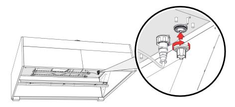
To remove the UV lamp from the canopy extraction chamber, open the lamp fixing clips by turning its screw fastener counterclockwise, and then carefully remove the UV lamp from the canopy extraction chamber.
