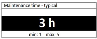
Enter the *Maintenance time – typical* view and using the control knob by turning it choose a value between 1-5. Once you have chosen a suitable value press the OK button to confirm this.
