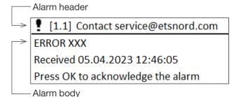
In most alarm cases you will need to contact the ETS NORD technician to determine the problem and how to fix it. In such a case the alarm will display the contact information at the top of the alarm notice and the error code in the body.
