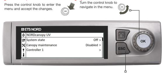
Press ESC button to cancel changes or move back to previous menu. Holding the key down for a few seconds of time returns the controller to its basic mode. The display shows the basic view, the background light dims.
